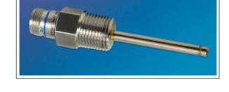
ETL-11-250 Series transducers are miniature, threaded flush instruments. The sensing sub-assembly is protected from mechanical damage by a "B" screen which has been shown to have minimal influence on the frequency response of the sensor. The ETL Series uses Kulite's Patented Leadless Technology. Incorporation
